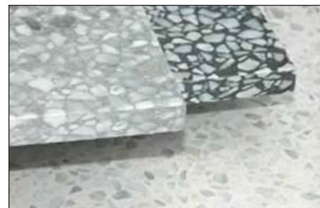
Figure 7: Different types of terrazzo floors
